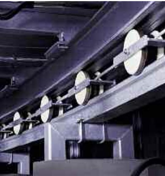
Ruggedly designed roller carriage is virtually maintenance free — no bearings or lubrication required.
